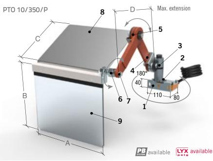
Specific multi-adjustable item to be installed on the longitudinal carriage.
