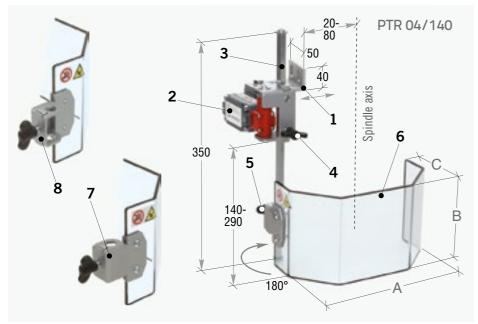
Small item, the only one with a double shield adjustment. Suitable to be used on drills, bench drills and similar machines.
