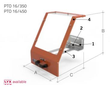
Swinging opening safety guard with double arm for the operator protection during working. Protects the operator from direct contact with rotating components of the chuck and from the projection of shavings and lubricant-coolant. Attachable in front of the longitudinal carriage. The shield is completely adjustable and, thanks to its configuration, allows the perfect view of the workpiece also from above.
