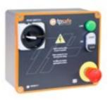
Electrical box for small dimension machines (example: sanders, grinders, drills and radial drills or small disc miter saws), made in die-cast aluminum case. Complete with general switch, no. 2 contactors, safety thermal relay with automatic reset, 400/24 VAC transformer, electronic motor brake device with DC injection (Exclusive Tecno Più), no. 4 fuses, double emergency mushroom-shaped pushbutton, start-stop button with motor start warning light and voltage warning light.
