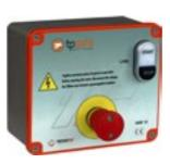
Electrical box for generic machines made in die-cast aluminum case. Complete with contactor, transformer 400/24 VAC, no. 2 fuses to protect the auxiliary circuits, emergency mushroom-shaped and start-stop pushbuttons, with voltage warning light and safety thermal relay. Panel for machines with Max absorption = 5KW/400V, IP65
