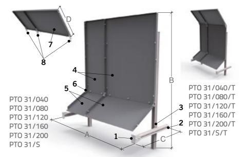
Modular system for rear protection and for shavings containment. Made of rapid release panels. To be fixed on the lower part of the base.
