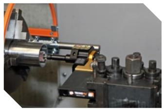
Grinding the inner surface.
