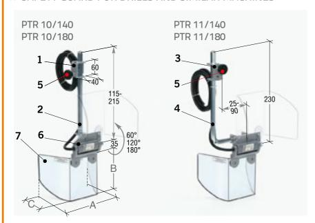
New item proposed with double fixing system, supported by adjustable hexagonal arms. Equipped with microswitch integrated in the rotation hinge.
