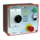
Electrical box for generic machines made in die-cast aluminum case, equipped with protection against short circuits and power overloads. Complete with magnetothermic motor protection general safety switch, prepared for padlock closure, contactor, 400/24 VAC transformer, no. 2 fuses to protect the auxiliary circuits, emergency mushroom-shaped pushbutton and start-stop pushbutton, with voltage warning light. Panel for machines with Max absorption = 7,5KW/400V, IP65.
