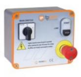
Kit for generic machines made in die-cast aluminum case. Complete with contactor, transformer 400/24 VAC, no. 2 fuses to protect the auxiliary circuits, emergency mushroom-shaped and startstop pushbuttons, with voltage warning light, general switch and safety thermal relay. Panel for machines with Max absorption = 5KW, at a voltage of 400V, IP65
