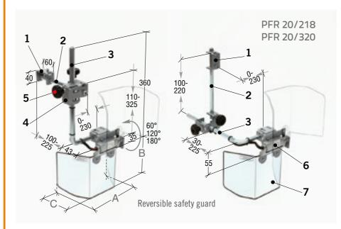
Exclusive item supported by adjustable hexagonal arms. Equipped with vertical opening shield, with microswitch integrated in the rotation hinge.
