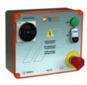
Electrical panel for generic machines with star/delta starting, in die-cast aluminum case. Complete with no. 2 contactors, 400/24 VAC transformer, timer for Star => Delta transition, no. 2 auxiliary circuit protection fuses, emergency mushroom-shaped and start-stop pushbutton, with voltage warning light, general safety prepared for padlock closure. Panel for machines with Max absorption = 5KW/400V, IP65.
