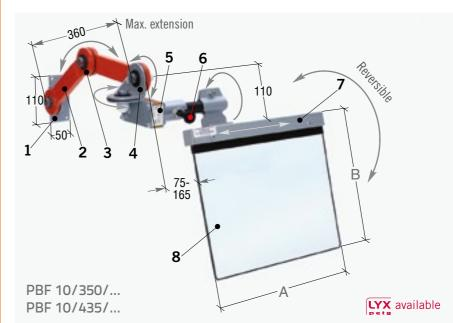
Universal rubbing articulated arms guard, with reversible opening direction. Practical and immediately adjustable. Designed for frequent changes of operation.
