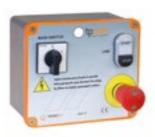
Electrical box for generic machines made in die-cast aluminum case. Complete with contactor, transformer 400/24 VAC, no. 2 fuses to protect the auxiliary circuits, emergency mushroom-shaped and start-stop pushbuttons, with voltage warning light and general switch. Panel for machines with Max absorption = 5KW/400V, IP 65
