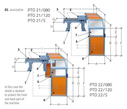
Sliding shield for big dimension lathe, designed to be fixed on the machine head and on the ground, making the whole structure of the guard stable.
