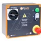
Electrical box for small dimension machines (example: sanders, grinders or small disc miter saws) made in die-cast aluminum case. Complete with general switch, no. 2 contactors, 400/24 VAC transformer, electronic motor brake device with DC injection (Exclusive Tecno Più), no. 4 fuses. emergency mushroom-shaped pushbutton, start-stop button with motor start warning light and voltage warning light.
