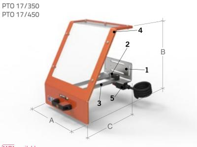
Swinging opening safety guard with double arm for the operator protection during working. Protects the operator from direct contact with rotating components of the chuck and from the projection of shavings and lubricant-coolant. Attachable in front of the longitudinal carriage. The shield is completely adjustable and, thanks to its configuration, allows the perfect view of the workpiece also from above.
