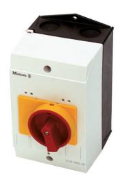
Kit for direct control of Simple Machines (e.g.: grinders). It consists of: thermoplastic case with three-pole magnetothermic safety switch with minimum voltage coil, not suitable for connection with any safety microswitches of guards and/or pushbuttons as it has not a very low voltage circuit (e.g.: 24 V). Prepared for padlock closure. Panel for machines with Max absorption = 7,5KW at a voltage of 400V.
