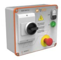
Kit for generic machines made in die-cast aluminum case, equipped with protection against short circuits and power overloads. Complete with magnetothermic motor protection general safety switch, prepared for padlock, contactor, 400/24 VAC transformer, n. 2 fuses to protect the auxiliary circuits, emergency mushroom-shaped pushbutton and start-stop pushbutton, with voltage warning light. Panel for machines with Max absorption = 7,5KW.
