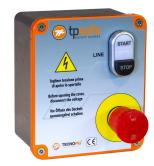
Kit for generic machines made in die-cast aluminum case. Complete with contactor, transformer 400/24 VAC, n. 2 fuses to protect the auxiliary circuits, emergency mushroom-shaped pushbutton and start-stop pushbutton, with voltage warning light. Panel for machines with Max absorption = 5KW, at a voltage of 400V.
