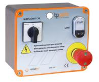
Kit for generic machines made in die-cast aluminum case. Complete with contactor, transformer 400/24 VAC, n. 2 fuses to protect the auxiliary circuits, emergency mushroom-shaped pushbutton and start-stop pushbutton, with voltage warning light and general switch. Panel for machines with Max absorption = 5KW, at a voltage of 400V.
