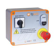
Kit for generic machines made in die-cast aluminum case. Complete with contactor, transformer 400/24 VAC, n. 2 fuses to protect the auxiliary circuits, emergency mushroom-shaped pushbutton and start-stop pushbutton, with voltage warning light, general switch and safety thermal relay. Panel for machines with Max absorption = 5KW, at a voltage of 400V.
