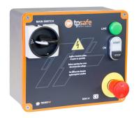
Kit for small dimension machines (example: sanders, grinders or small disc miter saws) made in diecast aluminum case. Complete with general switch, n. 2 contactors, 400/24 VAC transformer, **electronic motor brake device with DC injection (Exclusive Tecno Più),** n. 4 fuses, emergency mushroom-shaped pushbutton, start-stop button with motor start warning light and voltage warning light.
